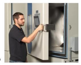
risk for an explosion. This is due to the fact that the standard nichrome wire heater used in most chambers can exceed 1000°F surface temperature. For this type of application temperature limited sheath heaters must be used at a minimum. Depending on the application, a classified explosion proof chamber may be required. There are many scenarios which could be used for examples, but the bottom line is to make sure you have given your chamber manufacturer all the details of your tests.
