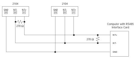
**Note:** 270  $\Omega$  resistors recommended across receive line on computer and last controller.
