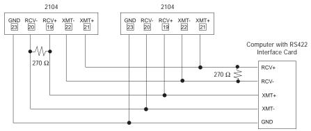
Note: 270  $\Omega$  resistors recommended across receive line on computer and last controller.
