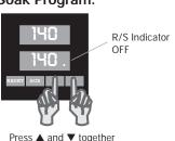
▼ and ▲ together (Stop Pushbutton) return the Ramp/Soak program to the Standby setpoint.
