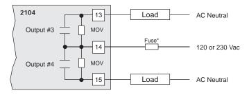
\* Fuse should be sized for the combined current of Output #3 and #4.
