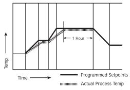
Guaranteed Soak is enabled on the ¬SP9 PASE by setting the differential band to a value greater than 0. It is adjustable from 1°F to the sensor span.
