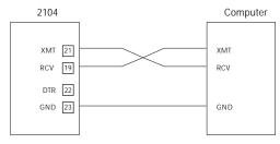
Note: The DTR output is always enabled when the 2104 power is on.
