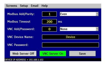
Touch the address entry field for the "Modbus Add/Parity" settings and enter the desired address for the controller on the network. The address entered here, will correspond to the address (device) number in EZ-View. In order to view the controller in EZ-View, the corresponding device address in EZ-View must be configured to match the EZT and be enabled under "Device Setup" in EZ-View.
