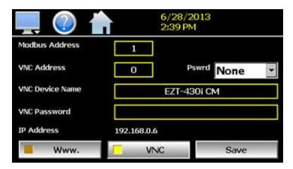
Touch the Modbus Address entry field and enter the desired address for the controller on the network. The address entered here, will correspond to the address (device) number in EZ-View. In order to view the controller in EZ-View, the corresponding device address in EZ-View must be configured to match the EZT-430i CM and be enabled under "Device Setup" in EZ-View.
