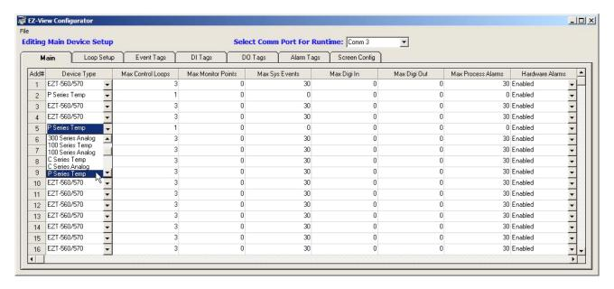
The **Device Type** controller selections include the EZT-560/570, EZT-430i-LC, EZT-430i-CM, 300 Series Temp and 300 Series Analog, 100 Series Temp and 100 Series Analog, C Series Temp and C Series Analog, P Series Temp and P Series Analog and L91/L41 Temp and L91/L41 Analog. IO Module selections include the IO-8IIA(mA), the IO-8AIVS(V), the IO-8TCS (T/C-C) and (T/C-F), and the IO-6RTD (RTD-C) and (RTD-F).
