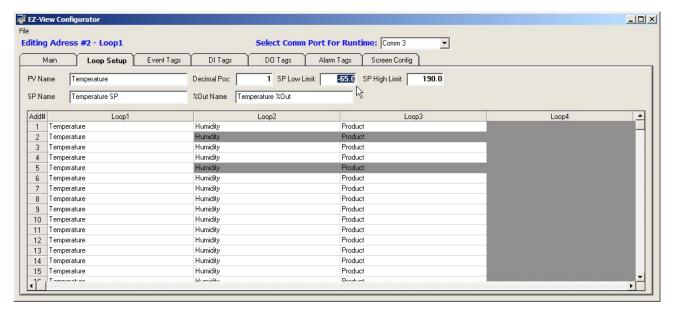
**NOTE:** If you do not enter a description for a field, i.e., the loop control PV Name or SP Name for example, the field will not be shown in EZ-View and you will be unable to view the data, data log it or change its value, even though you enabled the loop on the Main tab.
