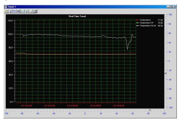
The -100 to +100 scales at the bottom and to the right of the trend are for scale/time compression/expansion. This is an analysis tool to "zero" in on specific data in the trend. It's a zoom in/out adjustment for the trend scale and time scale.
