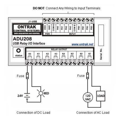
**WARNING:** It is the responsibility of the end user to properly install and wire the relay outputs of the ADU208 relay card according to all applicable electrical codes. The use of 120Vac power poses a shock hazard due to exposed relay terminals. It is recommended that a Class 2, 24V power supply be used to power indicator lamps, audible alarms, etc., as required.
