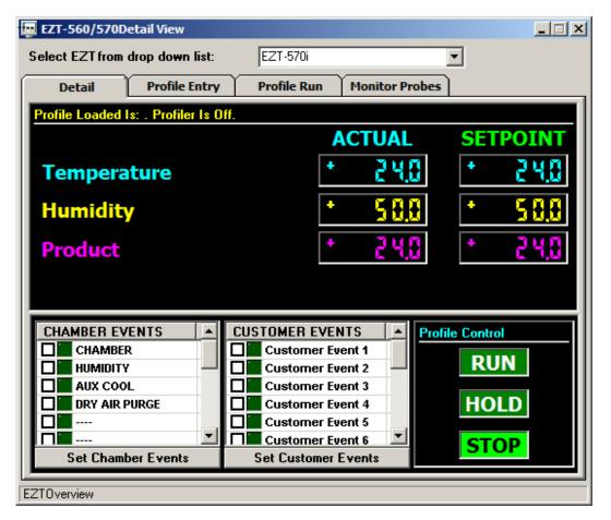
To change a loop's setpoint, click on the current setpoint and enter the desired value. EZ-View automatically keeps track of each loop's min/max setpoint limits as entered in the configurator, so if the user enters a value that exceeds the minimum or maximum allowed setpoint, the value will be coerced to the corresponding limit value.
