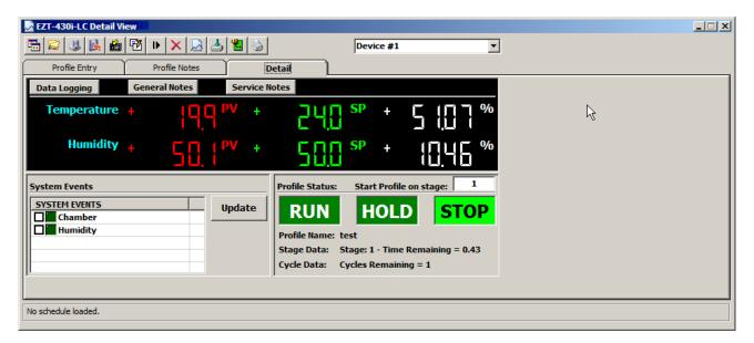
To change a loop setpoint, click on the current setpoint in the main digital display area and enter the desired value. EZ-View automatically keeps track of each loop's min/max setpoint limits as entered in the configurator, so if the user enters a value that exceeds the minimum or maximum allowed setpoint, the value will be coerced to the corresponding limit value.
