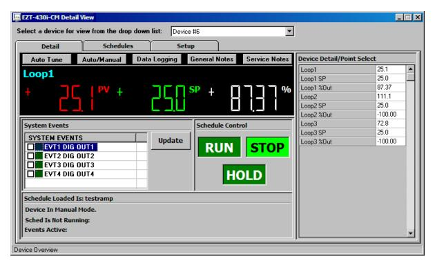
The main digital display window allows the user to select and control each loop of the EZT-430i CM. The selected loop will have its tagname shown in the top left of the window. To select other control loops, simply click on one of the tagnames associated with the desired loop in the Device Detail/Point Select list box on the right of the screen.
