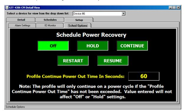
Select **OFF** to have the EZT-430i CM default to the off state on power-up. If a profile was running when power was lost, the profile will be stopped. In addition, all system events will be turned off. Note that loop controls will continue with the profile's last set point value prior to power loss with loop control outputs active (ON).
