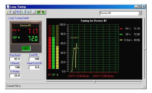
The screen has fields for viewing and adjusting proportional band, reset, rate, cooling PB and deadband (gap between heat and cool control). The drop down list box located at the top right of the loop tuning window is used to select any single loop control in the system to work with.
