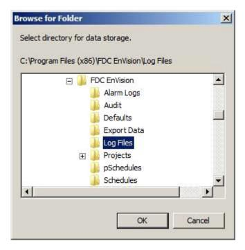
**NOTE:** In order for EZ-View to begin using the new storage path, the logging setup for the device (or system log) must first be saved. This prevents he storage path from being altered while logging is currently active for the device or system.
